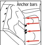
LATCH means Lower Anchors and Tethers for CHildren. Not all vehicles manufactured before September 2002 were equipped with LÄTĊH.
